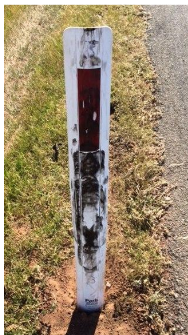
Figure 6, Post 3 after testing at 100km/h
